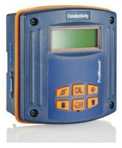
The 2-wire transmitter DMTa converts the following sensor signals into an interference-insensitive 4-20 mA analogue signal: pH, ORP, temperature, chlorine and conductivity.
