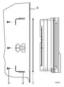
*Fig. 5: The material thickness of the control panel must be at least 2 mm to ensure secure fixing*
