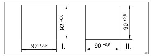
Fig. 16: Mounting - control panel installation DULCOMETER® D1Cc
