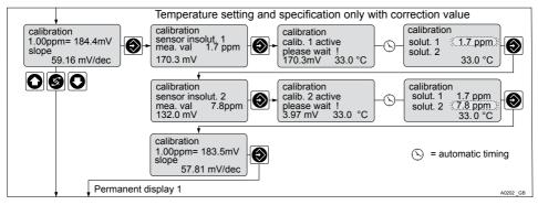
Fig. 45: Calibrating the fluoride sensor
