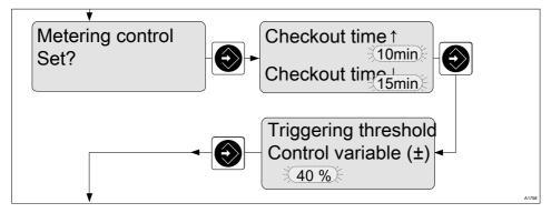
*Fig. 66: Metering time: Adjusting the checkout time and control variable triggering threshold.*
