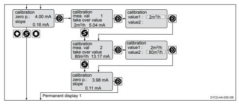
Fig. 52: Two point calibration menu / shown with flow as the measured variable and the measuring range  $0...100 \text{ m}^3/\text{h}$
