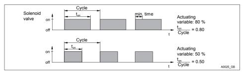
Fig. 60: Solenoid valves
