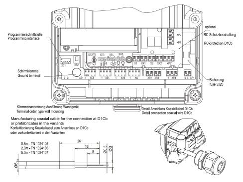
Fig. 9: Preparation of coaxial cable
