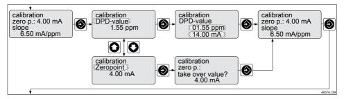
Fig. 38: Calibration of All Amperometric Measured Variables
