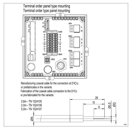
Fig. 18: Preparation of coaxial cable
