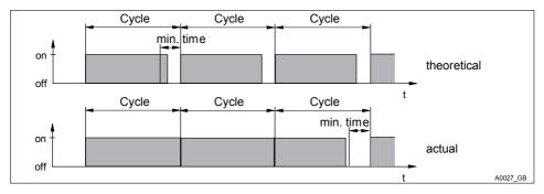
Fig. 62: Theoretical switching time > (cycle - min. time) and calculated switching time < cycle
