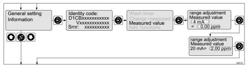
Fig. 72: Setting the measured value (for example "chlorine")
