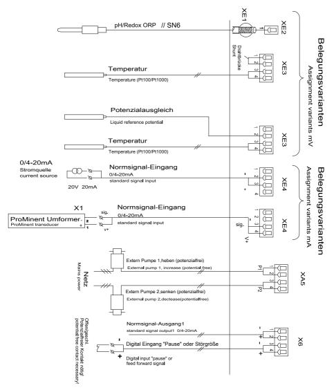
Fig. 12: Terminal diagram with assignment options 2
