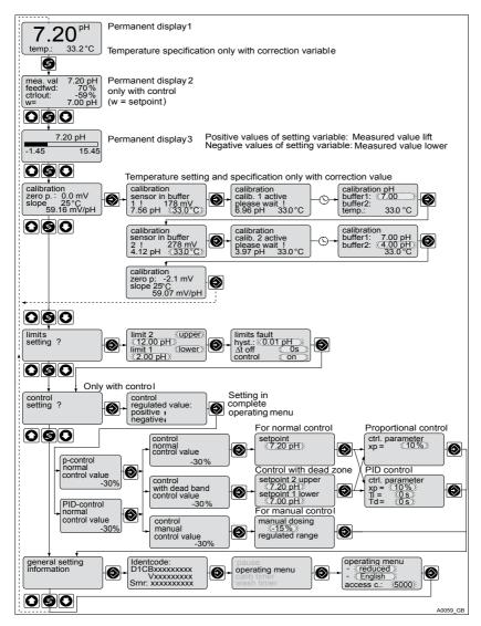
Fig. 41: Reduced pH / redox / fluoride operating menu (shown with the example of pH)
