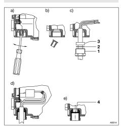
Fig. 7: Punching out the threaded holes
