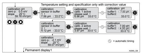
Fig. 43: Calibration of pH sensors
