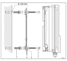
Fig. 3: Fixing material for wall mounting
