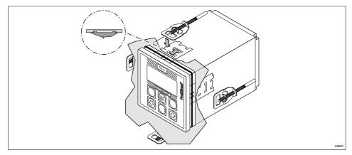
Fig. 17: Screw the studs forward
