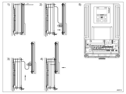
Fig. 6: Opening the device
