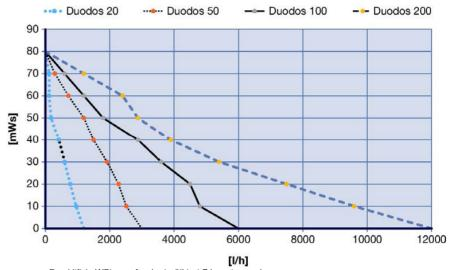
Feed lift (mWS) over feed rate (I/h) at 7 bar air supply
