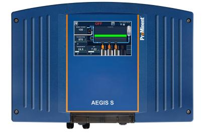
AEGIS S is an easy-to-use water treatment controller for evaporative cooling systems. It is designed to keep the cooling process running reliably. AEGIS S measures conductivity and controls dosing of biocides and corrosion inhibitor, thus preventing biological growth and keeping pipelines and heat exchangers clean.
