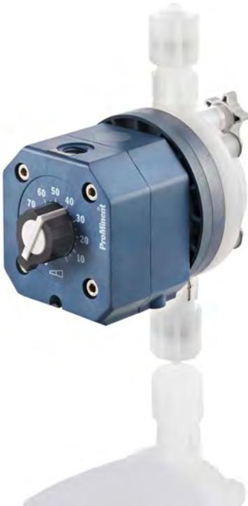
ProMinent® Pneumados is a pneumatically-operated metering pump. In contrast to solenoid-driven metering pumps, the metering stroke of this pump is effected by a pneumatically actuated diaphragm, the suction stroke by spring force.
