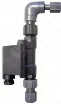
**Sample Water Low Flow Switch**, suitable for fitting to inlet connection on by-pass probe holder assembly, (8 x 5). Arranged to pause controller. This unit is fitted with opposing magnets that act like a spring so it can be mounted in any position. Supplied complete with fittings. Normally Open or Normally Closed contacts available.
