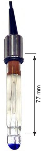
PROBE rH Peripheral Probe 3.5mm Platinum Band. 0-100°C HT3 glass Glass Body, Pinwick, Double Junction, SS Flared Cap, 10.0m Co-axial Cable, Pin Lug Connections.
