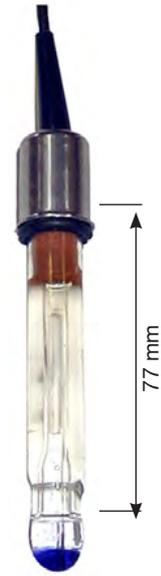
PROBE rH Peripheral Probe 3.5mm Platinum Band. 0-100°C HT3 glass Glass Body, Pinwick, Double Junction, SS Flared Cap, 10.0m Co-axial Cable, Pin Lug Connections.
