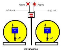
Twin Drum Scale & Control Unit (Digital) with alarm & 4-20 mA
