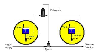
Note: All Ton mounting regulators, vertical & horizontal headers are fitted with 240V heaters. We suggest connection via a Residual Current Device (RCD) safety switch.
