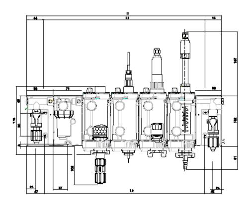
BAMa design example: BAMa\_EU\_1\_2\_1\_1\_X\_D\_D\_C\_1\_X\_00\_01\_00\_DE (with float flow control, e.g. for drinking water)
