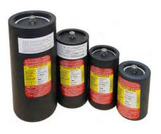
**Note:** Dampers are supplied uncharged & have to be filled according to the pressure in the system they will be installed in with either dry nitrogen or air. As a rule of thumb 70% of line pressure.
