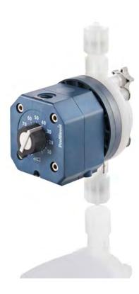
ProMinent® Pneumados is a pneumatically-operated metering pump. In contrast to solenoid-driven metering pumps, the metering stroke of this pump is effected by a pneumatically actuated diaphragm, the suction stroke by spring force.
