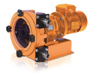
The peristaltic pump DULCOFLEX DFBa is designed for low and medium pump capacities of up to 800 l/h. Depending on application, the pump can be set for a back pressure of up to 8 bar.
