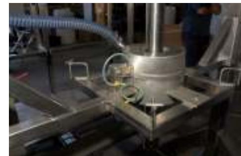
Bag clamp coupling With ring of vacuum
