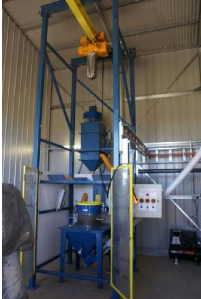
Bulk bag loader with crane and hoist unloading from the bottom of the bag
