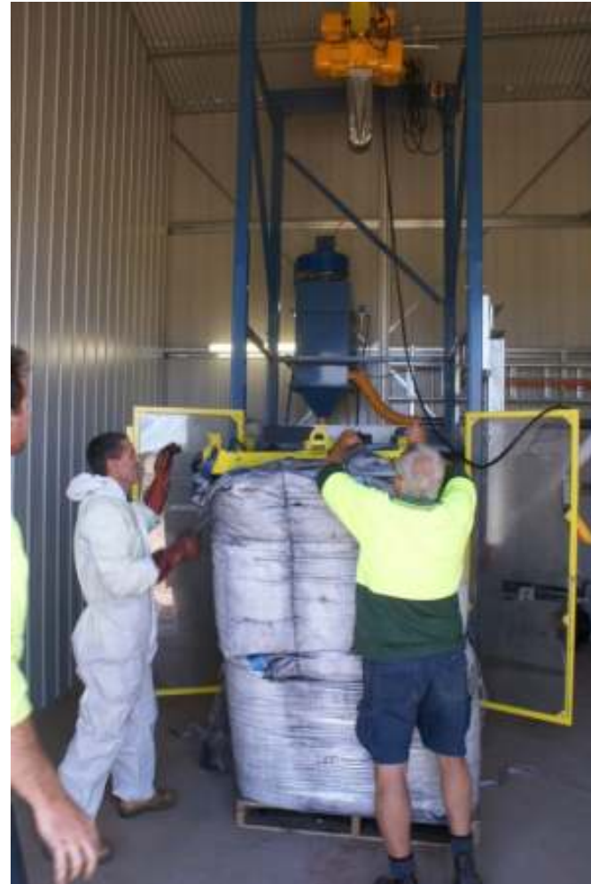
Bulk bag loader with crane and hoist unloading from the bottom of the bag
