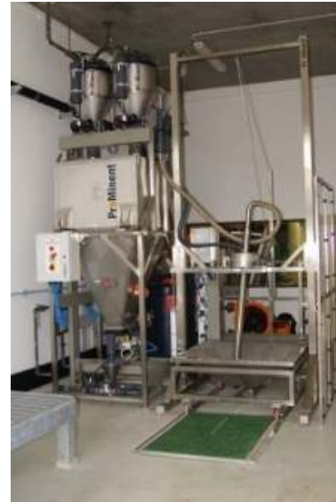
Vacuum loader from top of a bulk bag
