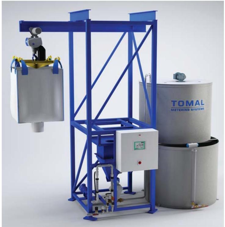
**Telfer beam stand** with an electrically operated lifting hoist. The chain hoist transports the big bag vertically and sideways to allow for easy positioning with the supplied pendant control. Limit switches and slip clutch are included as standard.
