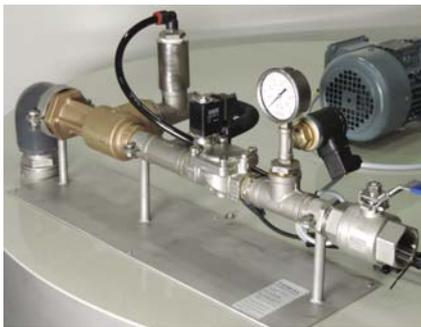
Inlet armatures including the high-effective injection nozzle.
