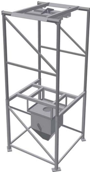
**Adjustable height big bag stand** includes a lifting yoke for handling by forklift or hoist. The operator lift the big bag into the stand and keep it hanging during the emptying. As the upper support is adjustable it gives a possibility to adapt different big bag sizes and have them stretched for optimized emptying.
