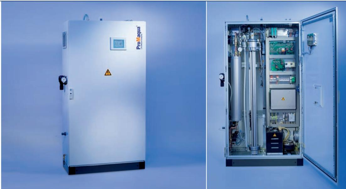
The ozone generating system OZONFILT®OZMa guarantees maximum operational safety and reliability at minimum operating costs. Depending on the version, the system produces ozone from compressed air or oxygen at a rate of 70 to 245 g per hour. Electronic power circuitry ensures a reproducible ozone quantity independent of power supply and pressure fluctuations. The electronics additionally provides full protection for all electrical components.
